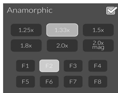
In this example, the user enabled the function "ANAMORPHIC" with the value 1.33x associating it to Function Button F2.
