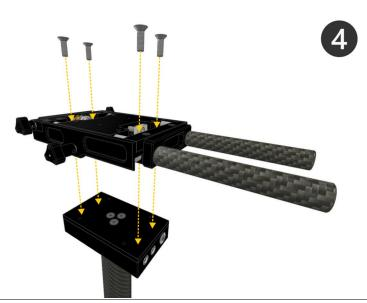
**Step 4**: Make sure the previously highlighted holes are aligned on the counter part on Matrix sled and insert the 4x M5 screws tighten them with Hex 3 key
